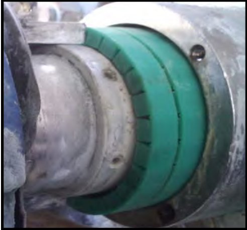
Place PCK as shown to compress each ring into the stuffing box.
