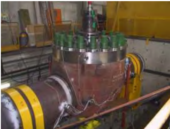
BT2 38 in. (950 mm) API 5000 cladded in all wetted parts during bending test.
