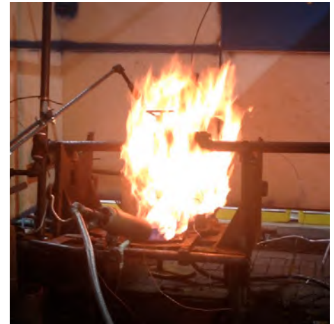
Fire test per API Spec 607 4th Edition.
